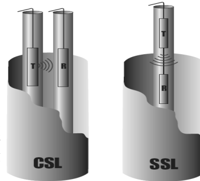
Test Arrangement for Cross-hole Sonic Logging CSL and Single-hole Sonic Logging SSL
